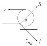
Let the angle between the radius to the point of contact with the step and the downward vertical be  $\theta$ , as shown.
